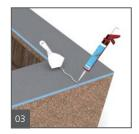
The wedi Building Panel is installed over the structure using modified thinset mortar. wedi Fasteners are additionally applied on vertical areas (1 per sq. ft.), no fasteners are used in horizontal areas. All seams, protrusions or fastener points must be waterproofed using wedi Joint Sealant.
