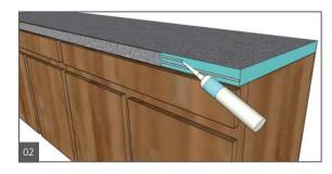
Apply wedi Joint Sealant and a strip wedi Building Panel in any thickness starting from 1/8" thick standard wedi Building Panels. This strip's cementitious coating side will allow you to better set small tile.
