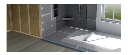
Extend your waterproofing from shower and tub areas into the whole bathroom with wedi Building Panels on your floor. Especially when installing floor level entry showers, a waterproof tile underlayment is needed in front of a shower entrance. wedi Building Panels can help you create both in one step: your waterproofing and tile underlayment as well.
