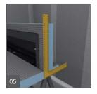
Make sure the Fundo Discreto is installed with a tight angle/ perpendicular to the shower base surface.
