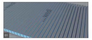
Create a series of cuts into the wedi Building Panels 1/2 the thickness of the panel deep. The distance between cuts depends on the tightness of the radius needed later. Use a circular saw for these cuts.
