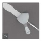
Seal all joints and fastener points using wedi Joint Sealant or wedi Sealing Tape. In dry areas, use wedi Self Adhesive Mesh Tape.
