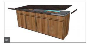
Install the large format, thin porcelain tile over the wedi Building Panel surface and edges using a modified thinset.
