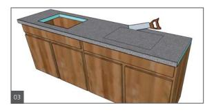
Cut out for the sink using a jigsaw or handsaw. As needed, recess cuts might be created with a utility knife or a router to accommodate recessed sinks. Cutting the holes may proceed before or after installation of large format, thin porcelain tile as indicated in step 05.
