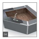
The tub deck can be tiled over immediately once the wedi board is installed, seams and possible fasteners and cut outs sealed and the thinset mortar has set up.
