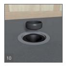
Set up the rubber caulking gasket (with the bevelled side up) around the 2" pipe in the subfloor. The rubber gasket must be flush with the upper end of the 2" ABS or PVC pipe. Do Not use any Lubricants.
