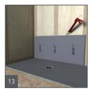
Push the wedi panel all the way into the channel of the shower base channel and its bead of sealant. Smooth out any pushed out sealant on inside seam using a putty knife. Fasten the panels directly to the studs starting 1 ft above the base and at a rate of 1 fastener per 1ft. One extra fastener is set into the seam to the next panel to crate a flush transition.
